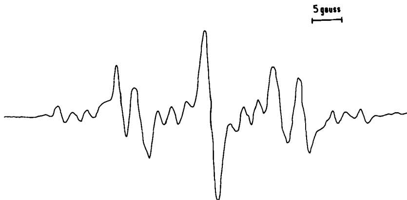
FIG. 5. ESR spectrum of vinyl chloride homopolymerization in DMF solution at 60°C after 23 min. Concentrations: monomer, 1.5 mole/liter; AIBN, 1.5 \times 10^{-2} mole/liter; tBuNO, 3 \times 10^{-3} mole/liter.
